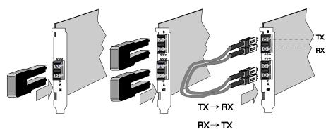
Figure 6. Setup for loopback testing
